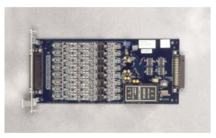
Onboard analog filters – similar to the analog filters on the iDSC 1816 – block unwanted high frequencies on each channel of the MSXB 048, shown here.
