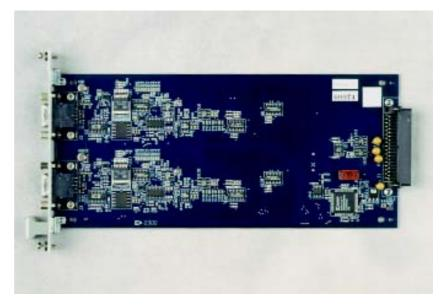
Key Component: 2-channel MSXB 044 board with 15-pin DB connectors shown at left
