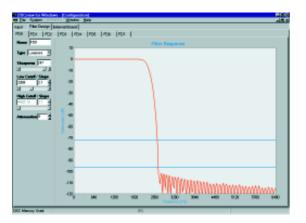
Onscreen sliders let you customize the filter on each channel. DSCview displays the characteristic curve in real time: like this one of a typical lowpass filter.
