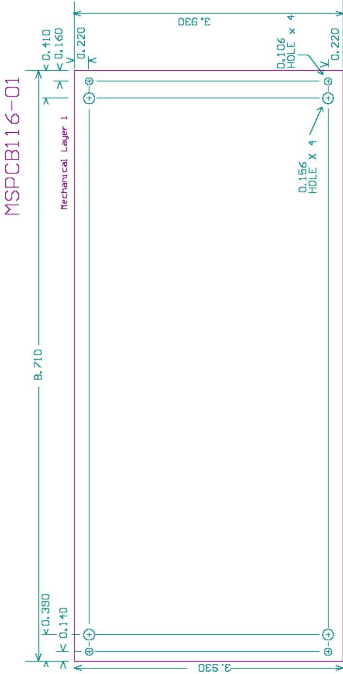
Figure 9. Dimensions of the Board.
