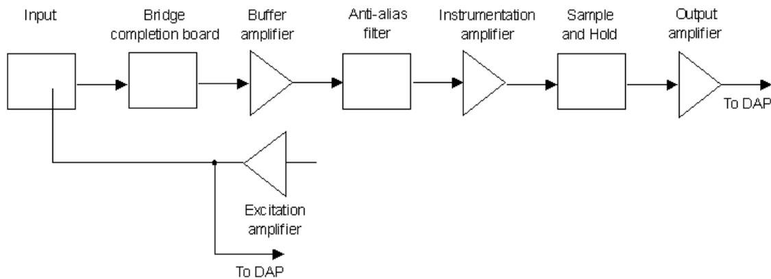
**Figure 1. MSXB066/067 Block Diagram.**
