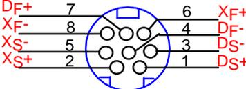
Figure 3. Sensor Input Connector.
