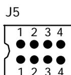
*Figure 6. Input Range Selection Header*
