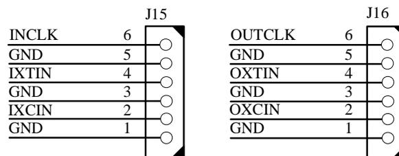
*Figure 8. External Clock and Trigger Signals*
