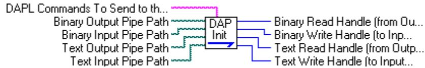
The DAPL Commands input accepts a LabVIEW string that contains DAPL commands for configuring a DAP. The remaining inputs normally are not used. They can be used if you would like to specify different communication pipes to open. If you are using more than one DAP it generally is best to make a copy of **DAP Init** and change the com pipe names from 'dap0' to 'dap1', 'dap2', etc. The output pins of **DAP Init** supply the handles that allow other functions to access the DAP communication pipes.
