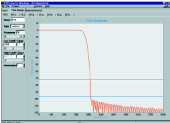
*Onscreen sliders let you customize the filter on each channel. DSCview displays the characteristic curve in real time: like this one of a typical lowpass filter.*
