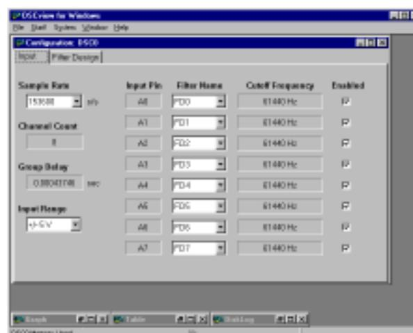
*Displayed properties include transition band cutoff frequencies for each channel, and group delay.*
