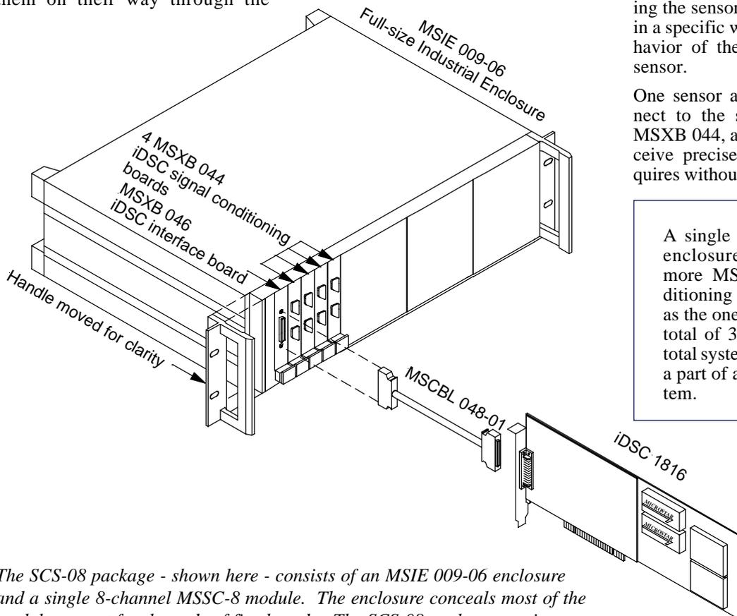
The SCS-08 package - shown here - consists of an MSIE 009-06 enclosure and a single 8-channel MSSC-8 module. The enclosure conceals most of the module, except for the ends of five boards. The SCS-08 package requires an MSCBL 048-01 cable to send conditioned signals to an iDSC 1816 anti-aliasing data acquisition board in a PC. It also requires another cable, not shown here, to carry power from the PC.
